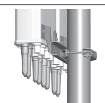
Recommended torque for M8 bolted connections: 20 Nm
